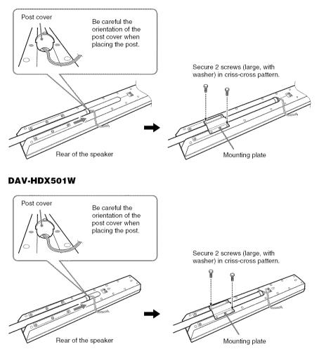
When securing the mounting plate, position the mounting plate depending on the desired height of the speaker.
